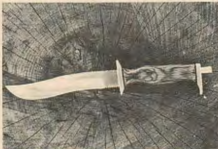
Custom fighting/concealment knife made by Mark Lahrman of Indianapolis, Ind. Knife has 440C stainless blade, micarta handle, stainless-steel mounts. Photo: Dan Fitzgerald
